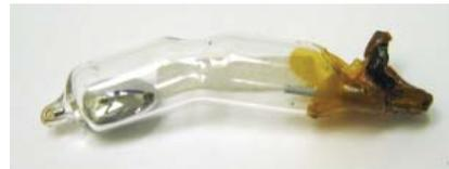
Mercury is used in devices today because of its excellent conductivity and high surface tension which allows it to roll freely. In a switch, for example, it makes or breaks electrical circuits signaling the furnace to heat or cool the air. Most people are not exposed to mercury because it is contained in a protective bulb. The harm is done when it breaks—often due to accidents when handling or after disposal.
